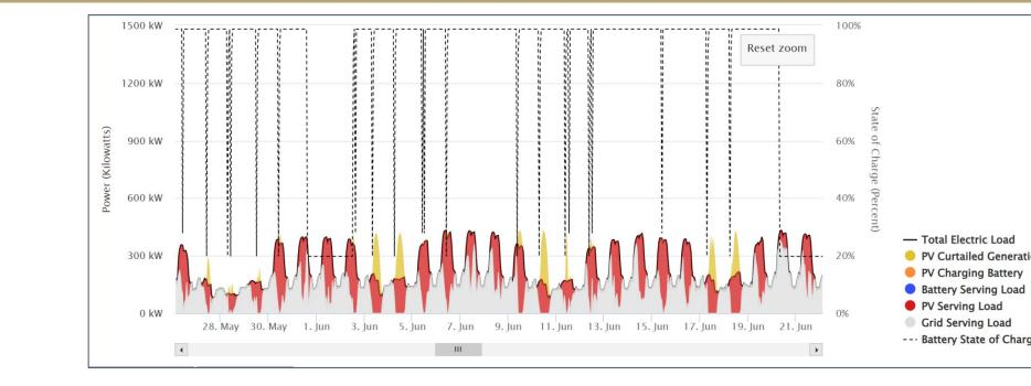
The REopt platform, run by NREL, evaluates the economic viability of distributed energy resources (DERs) for the microgrid, as well as strategies to mitigate the cost and achieve resiliency within the system. This simulation displays the potential load profile for the microgrid over 8760 hours, totaling one year in use.
